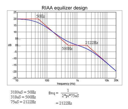
RIAA consist of 3 frequency corner which is 50Hz or time constant 3180uS , 500Hz 318uS , 2122Hz 75uS . the gain in 50hz and below is +20db which is 10 times gain, and below 20Khz is -20db which is attenuate 10 times. So the total different is 100 times from 50Hz below to 20Khz above.
