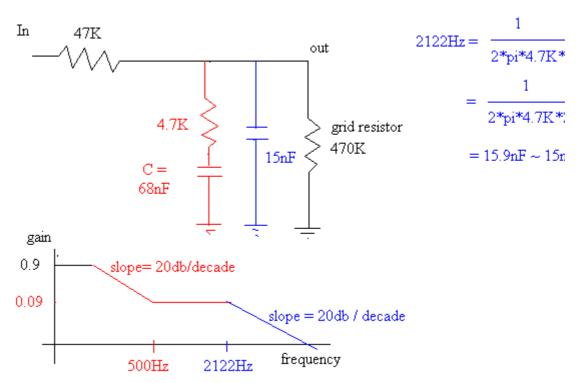
In order to complete another 75uS or 2122Hz corner , we need to add another capacitor , which is 15nF , which after 2122Hz the capacitor having XC as 4.7Khz and when above 2122Hz it start to go below 4.7K to cause further more attenuation until 20Khz and above it continue attenuate... since RIAA are only care up to 20Khz to make it simple we let it continue attenuate...
