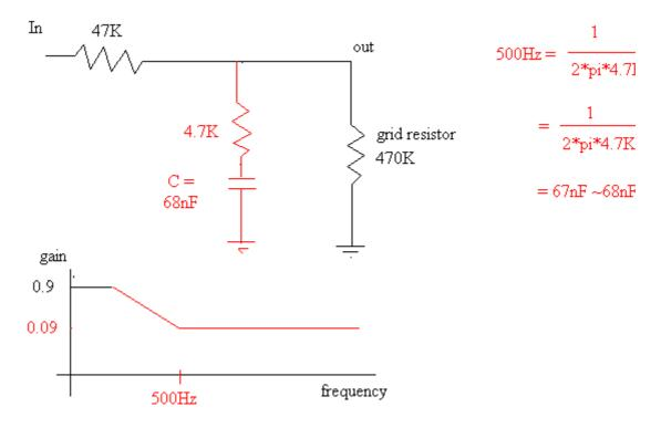
By adding a Capacitor when 500Hz have equal XC of 4.7K so when above 500Hz is go into below 4.7K or close to 0, so meaning that before 500Hz the capacitor having higher value then XC , so this will cause the slope from 50Hz to 500Hz slowly attenuate the gain until it
