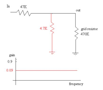
Since the RIAA at middle portion is 0db or and 50Hz below is +20db, because here all is passive component so there is not gain in here, so we offset +0db at 50Hz below , and 500Hz above is -20db , so which is attenuate 10times, so 0.9 to 0.09 gain , by adding 4.7K ohm resistor there.
