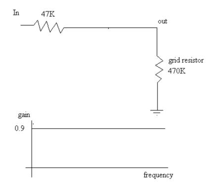
The grid resistor is the Rg1 for next tube , the 47K is just a beginning resistor , we cant choice too high it will have more attenutation versus 470K, if we choice too low since the tube having output impedance will series up with it and cause the frequency more depanding on tube then 47K. So for starting i assume the tube output impedance is much more smaller then
